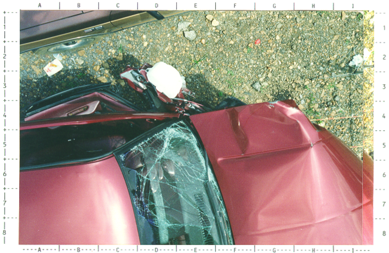
# 67 -- Overhead left front view of damage to '88 Chevrolet C-1500 pick-up; NOTE: stress cracks to left windshield
